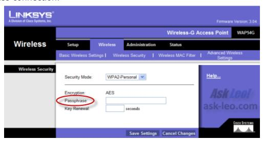
First: use WPA, not WEP. WEP encryption turns out to be easily crackable.
