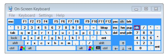
The on screen keyboard application is a "virtual" keyboard. It effectively has its own device driver, and to Windows "looks like" a real keyboard. As a result, the keystrokes it sends onto Windows can quite easily be captured by the same key logging software that's capturing keystrokes from the real keyboard, if that key logger has installed itself into the proper place.
